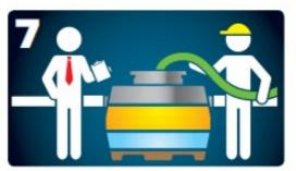
Observe pumper contractor work to ensure interceptor is fully pumped out, properly cleaned and in good condition.
