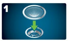
Use debris screens in all floor and sink drains. Regularly empty screens into trash.
