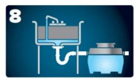
Make sure to run sinks to refill unit with cold water after pump-out.
